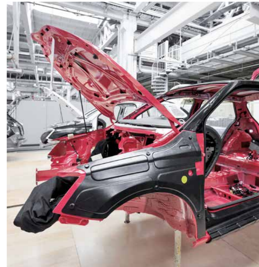
Figure: Components, assemblies, engines and gearboxes are all brought together during final assembly.
